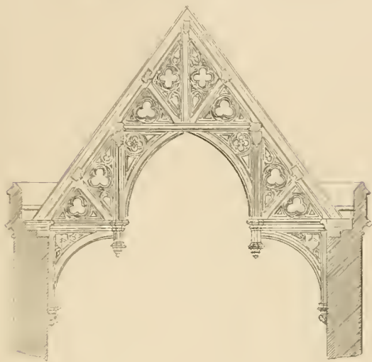
ANTIENT ROOF WITH THE FRAMING MADE ORNAMENTAL FIG. 1
